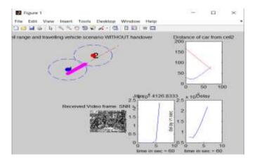
Fig.11Received Video, Delay and Jitter Graph when Handover not executed
